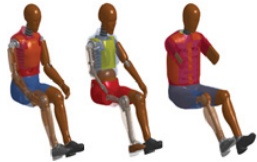
(left to right) Hybrid III 50 th male, Hybrid III 5 th female and WorldSID 50 th are commonly used dummy models.
