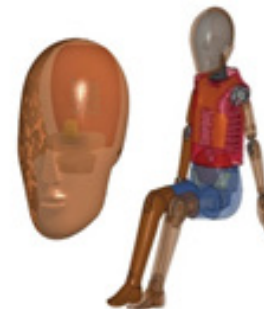
Other dummy models include Free Motion Headform (left) and Hybrid III 6-year-old (right).
