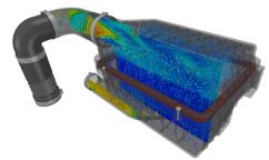
Discovery accounts for porous media to evaluate porous materials such as filters, screens and perforated plates within a product design.
