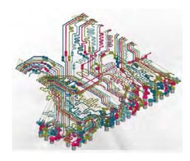
**SIwave – DC:** Engineers from Sarcina Technology LLC used Ansys SIwave to extract DDR3 electrical models for both a PCB and its daughter card to analyze the performance of application-specific ICs used in Big Data applications and the Internet of Things.
