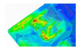
Current flow and thermal analysis simulations once performed separately can be combined in a multiphysics-based board-level electrothermal cosimulation via link-age between Slwave and Ansys Icepak.
