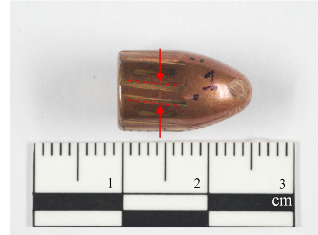
Deformed bullet after shooting by real shot
